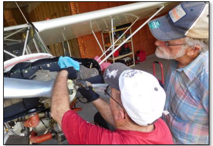
Eric Staton supervised while Mark Thoman safety wired the bolts.
