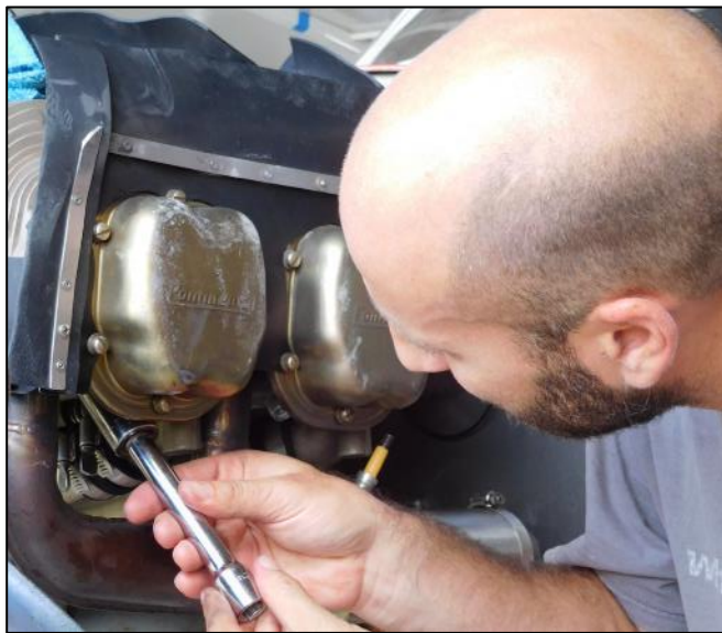
Chris Montefusco reinstalled the spark plugs.
