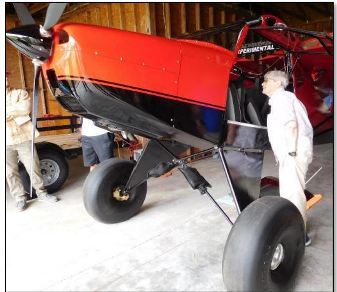
Wade's Highlander has a pair of 29-inch diameter rough terrain tires mounted on a landing gear structure that looks indestructible. The company engineer claims that you can drag the airplane, at near stall speeds, to the runway, and at an altitude of five feet, just chop the throttle and drop to the ground. With the brakes ON! That's quite a landing technique!
