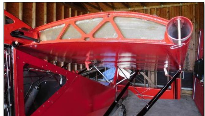
Wade's aircraft also is equipped with an ingeniously simple wing fold mechanism. There is a hinge mounted on the rear spar, and a vertical pin in the main spar, both located just outside of the fuselage section. To fold the aircraft a small panel on the top of the aircraft, just aft of
