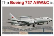
The **Boeing 737 AEW&C** is a twin-engine airborne early warning and control aircraft based on the Boeing 737 Next Generation design. It is lighter than the 707-based Boeing E-3 Sentry, and has a fixed, active electronically scanned array radar antenna instead of a rotating one. It was designed for the Royal Australian Air Force (RAAF) under "Project Wedgetail" and designated E-7A Wedgetail.
