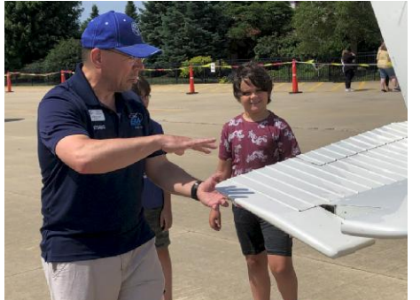
Dave Vancina explains the function of the elevator.
