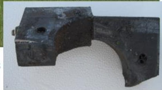
Fractured lower nose gear bearing
