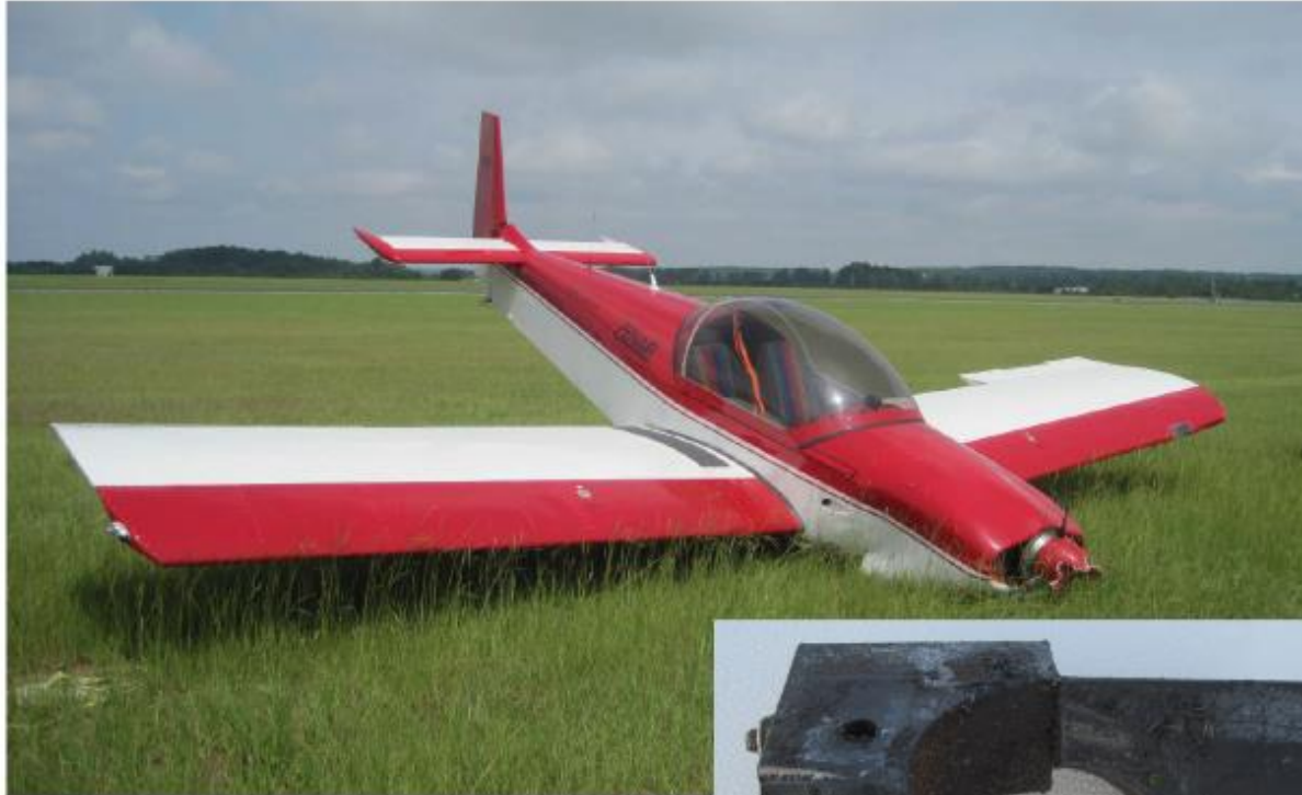
Fractured lower nose gear bearing
