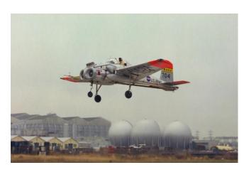
With ungainly proportions, Beechcraft wings and tail surfaces, and a primitive flight control computer strapped to the nose, the Bell X-14 was a decidedly unconventional X-plane. [Credit: NASA]
