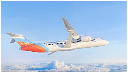
The Sustainable Flight Demonstrator project seeks to inform a potential new generation of more sustainable single-aisle aircraft – the workhorse of passenger airlines around the world. Boeing will work with NASA to build, test, and fly the X-66A, a full-scale demonstrator aircraft. The X-66A with extra-long, thin wings stabilized by diagonal struts, known as a Transonic Truss-Braced Wing concept.
