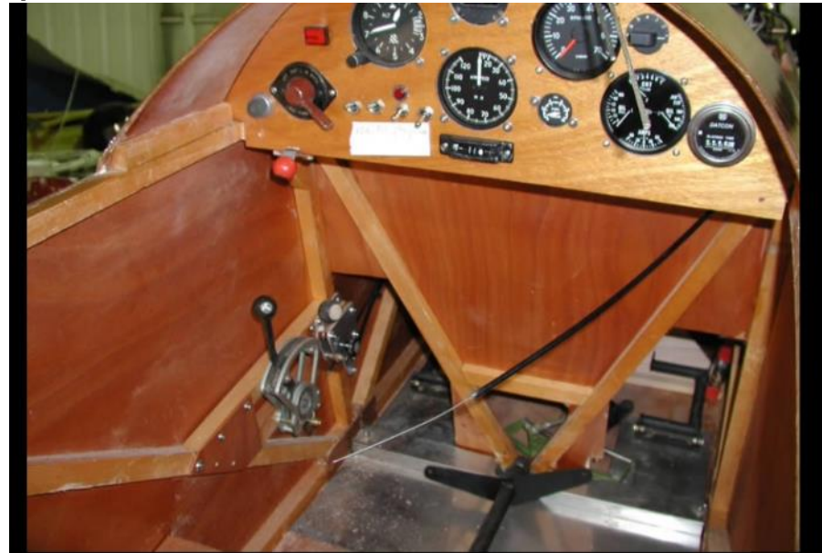
from left to right: Start button, A-9 mag and battery switch, red knob below is choke, red button above is battery warning light, altimeter, 4 switches are ignition, avionics, fuel pump w/ warning light and strobe, ASI, Compass, fuel press, tach, quad gauge is amps, oil press, oil temp, and CHT with rotary switch with probe on each cylinder. Hobbs meter. Below on left is throttle and small control ahead is carb heat. The cable hanging down not connected is fuel shutoff.
