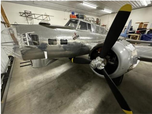
The engines are rated at 80 hp, but with no room for a prop speed reduction unit in the scaled-down cowlings, the engines are connected directly to the propellers, resulting in 60 hp at 3300 rpm, or a total of 240 hp. They burn about 4 gph each, for a total of 16, sipping from two tanks in the wings with a total
