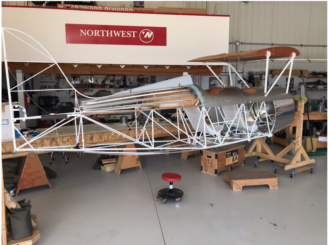
Wrapping up the sheet metal on the top of the fuselage.
