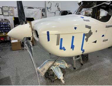
Propeller and spinner installed. Currently working on matching engine cowling up with proper clearances with spinner.
