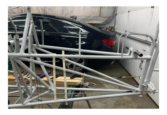
Next up was cleaning, inspecting, and repainting the rudder pedals control torque tube assy. Then installing and shimming so it all ran smoothly without binding.
