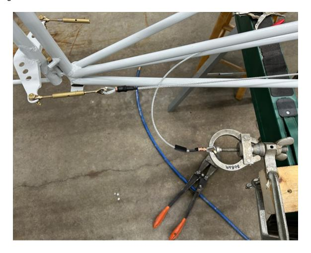
With the cables installed don't forget to measure where the cables will pass through the fabric in the future. Taking dimensions from the tan tape below.
