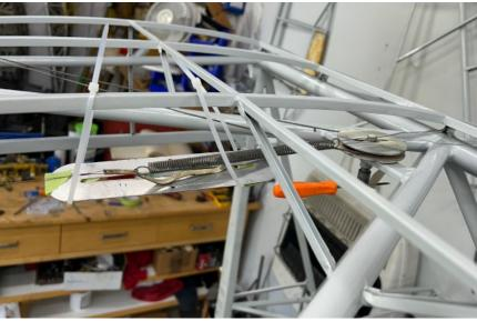
After that all the tail was installed and rigged after I cleaned up and inspected the tail brace wires.
