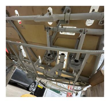
And finally, I made all new floor boards from 1/4" 5 ply Baltic birch, and then blasted and painted the bench seat frame.
