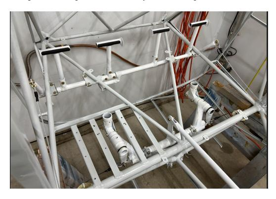
Next up was rebuilding and reinstalling the Scott brake master cylinders.
