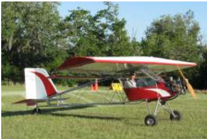
Photo 4 Anew part 103 ultralight at Sun n Fun this year. It is called the Backyard Flyer. The engine is common in many of the RV motor homes. It is used for the generator.
