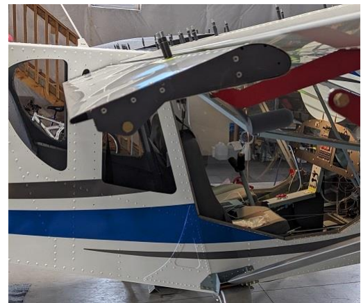
Right flap mounted to wing brackets and balanced
