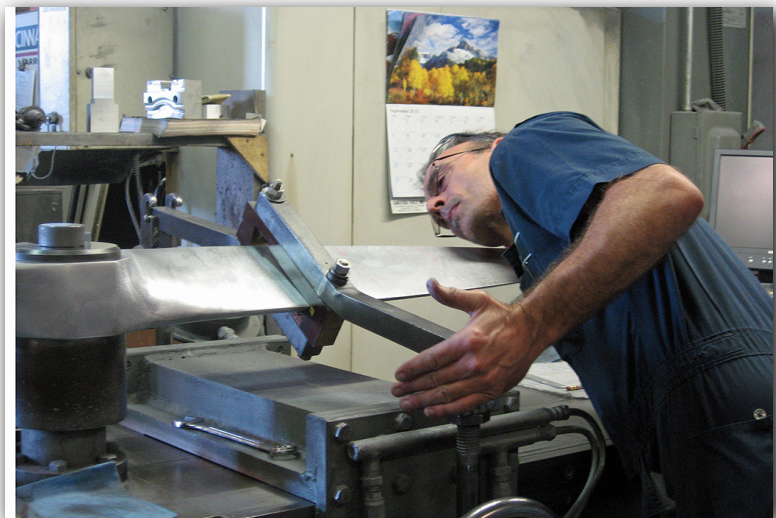
Figure 11 – Hydraulic blade bending machine – positioning the bender at the appropriate bending stations
