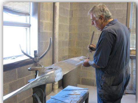
Figure 7 - Checking blade thickness
