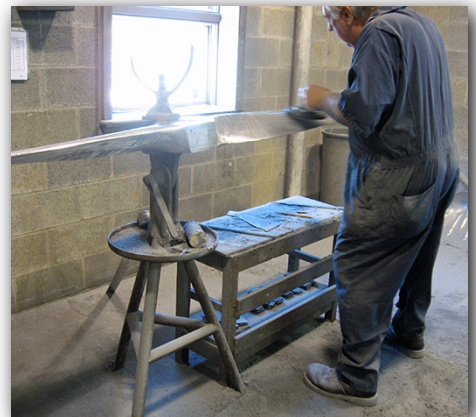
Figure 6 - Skilled worker using a sanding disk to shape the blade
