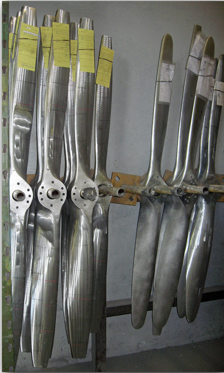
Figure 8 – Propellers between shaping and polishing operations
