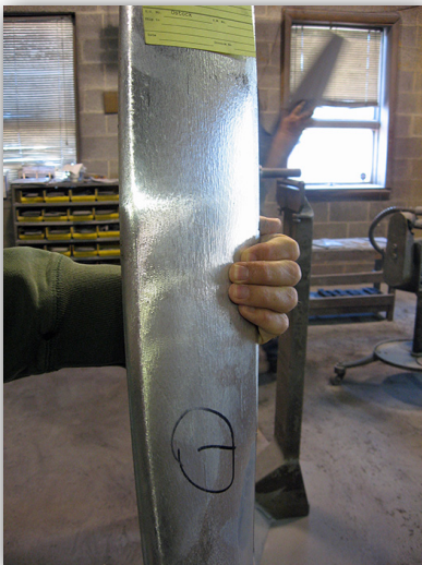
Figure 5 - NC Milled propeller blade, ready for manual smoothing
