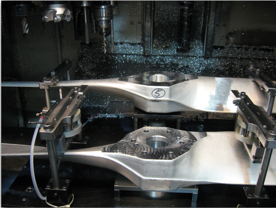
Figure 4 - Hub face milling
