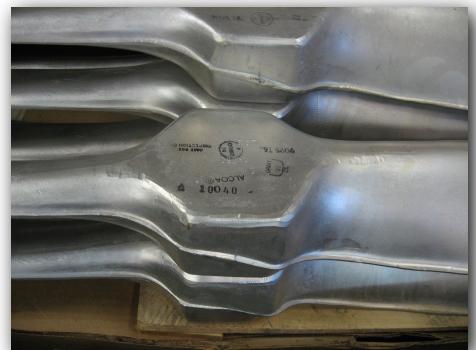
Figure 3 - Alcoa 2025 T6 forged propeller blanks
