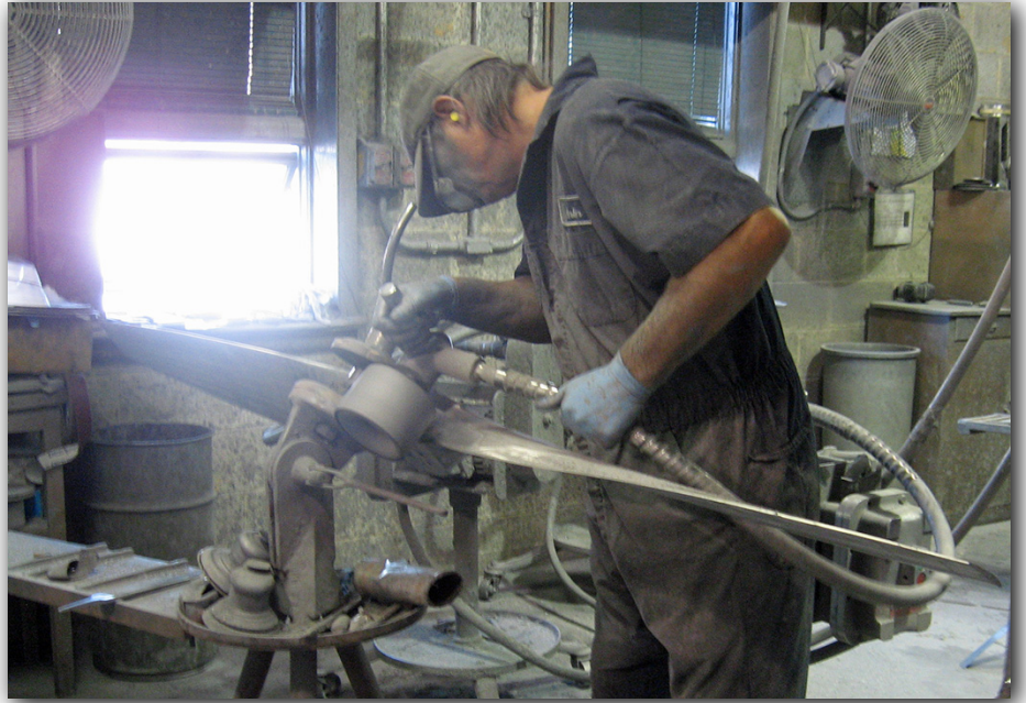
Figure 9 – Fine sanding/polishing of the blades.
