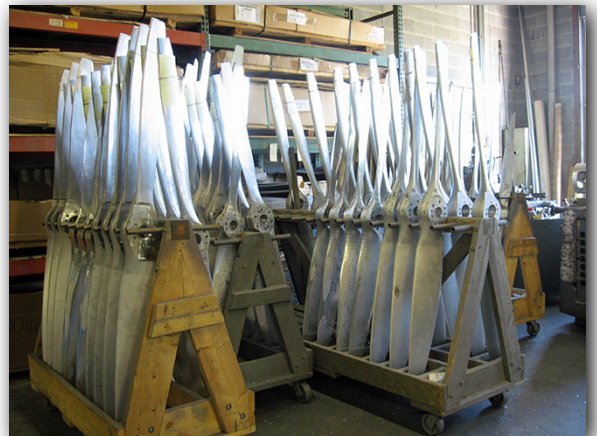
Figure 15 – Propeller overhaul - propeller blades with paint removed, and inspected.
