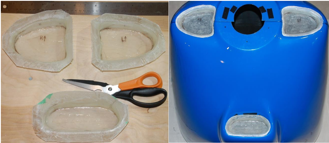
Figure 4. Roughly trimmed lips around each plug (left) and trial fit of the plugs into the cylinder head and oil cooler air intakes (right).
