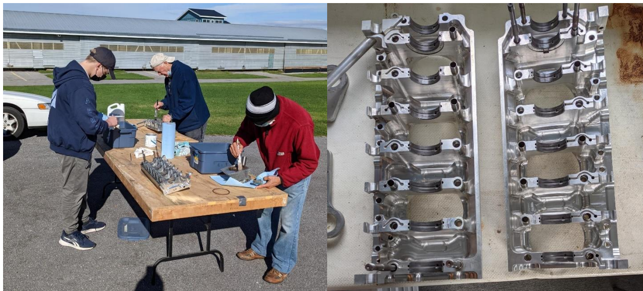
Figure 3. A warm workday at the Chapter 245 hangar in late October meant engine cleaning could be done outside (left), a shiny pair of crankcase halves after cleaning (right).
