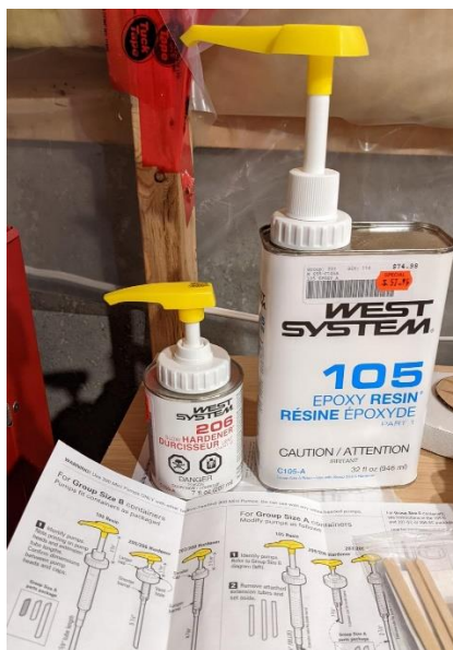
Figure 1. West Systems epoxy was used and purchased from The Chandlery in Ottawa along with 8 oz. fiberglass cloth, the metering pumps and stir sticks.
