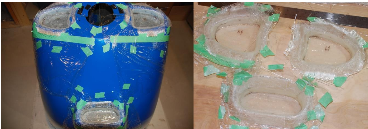
Figure 3. The cowl was protected with plastic wrap and the initial straight walled plugs were inserted. Fiberglass cloth was wrapped around the inside of each plug and overlapped the intake opening to create a rounded lip (left). The ragged plugs were removed after the second layer of cloth and resin had set (right).
