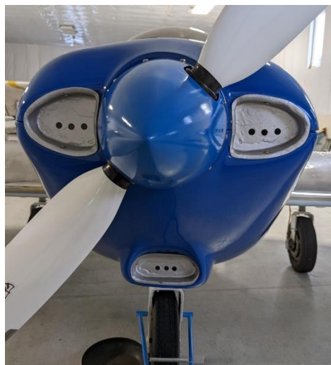
Figure 5. Air intake plugs installed and ready for first taxi tests with initial sets of air holes.
