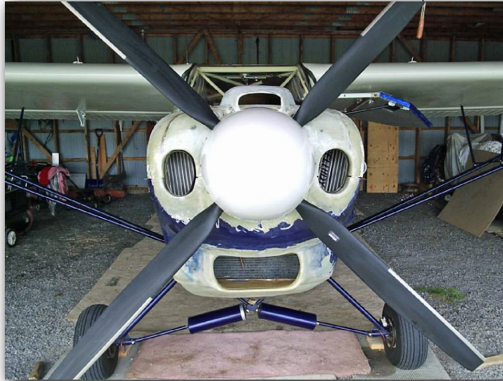
Photo 4: 2 Oil Coolers and Inlets
