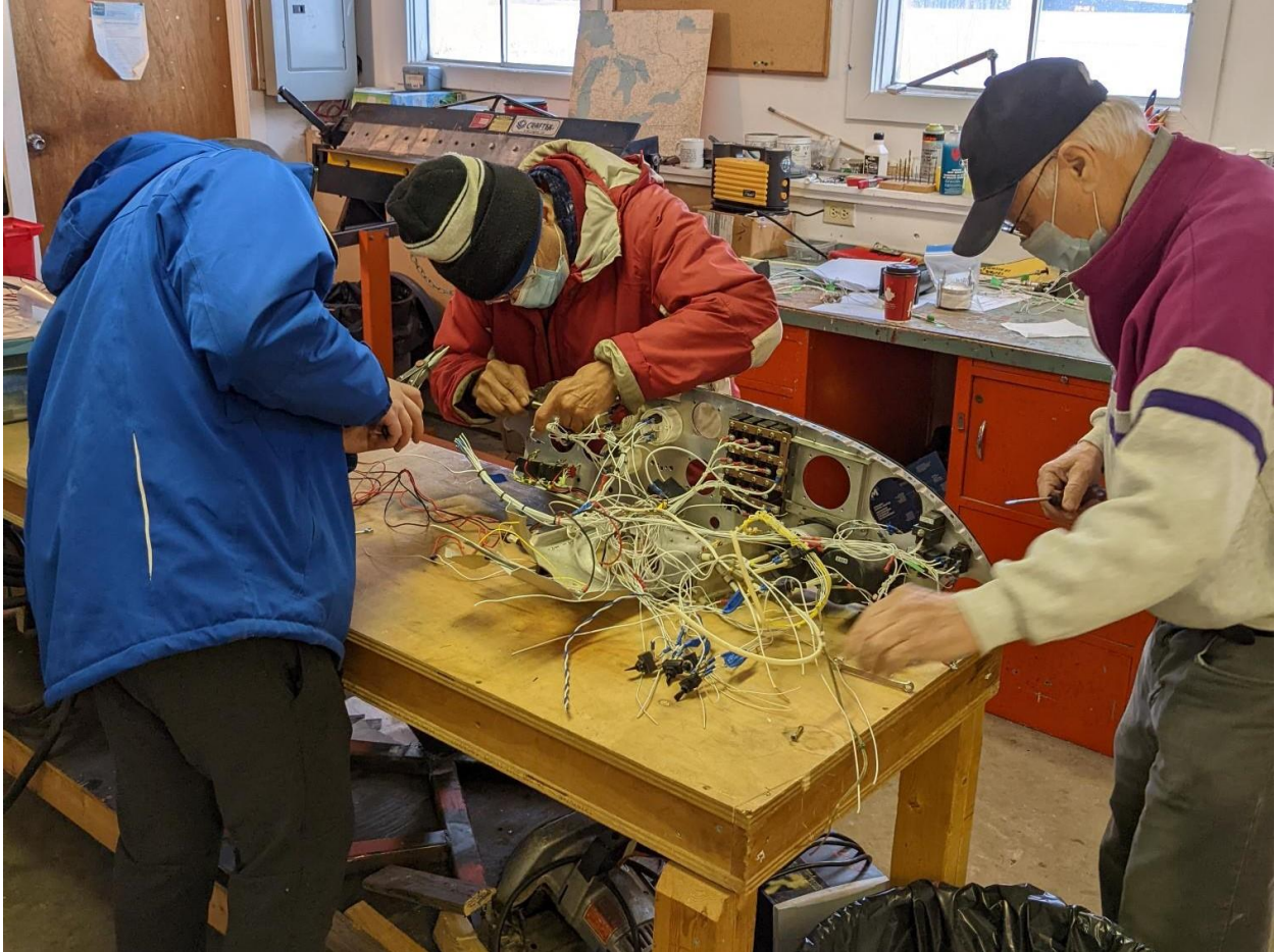
Figure 1. Colin, Edgar, and Yves (L to R) work on disassembling the old Zenair 601 panel. Instruments, switches, and circuit breakers were stripped back to their terminals, removed from the panel and then bagged for storage.
