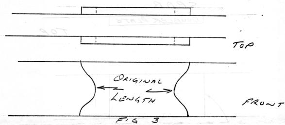
Please note that the minimum full flat length of the modified doubler plate must be no less than the original plans specified in doubler plate.
