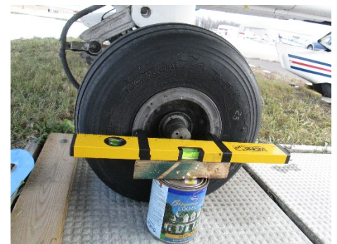
Figure 3 shows the level placed against the outer rim at the midpoint
