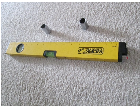
Figure 1 shows the laser level and two equal length sockets
