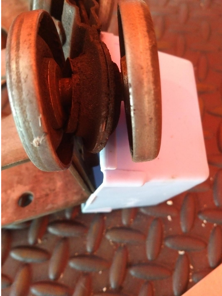
Photo 6: This end of this hanger, had its rollers vacate the holder so the shaft in this one was significantly worn down and ready to turn into another “wheel chock”.
