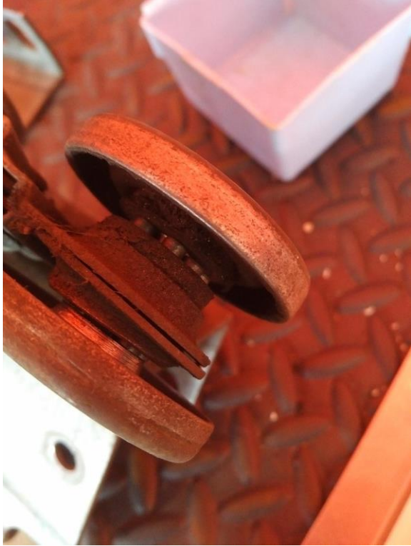
Photo 4: Deformed (bent) hanger brackets, bearings ready to begin to vacate the assembly
