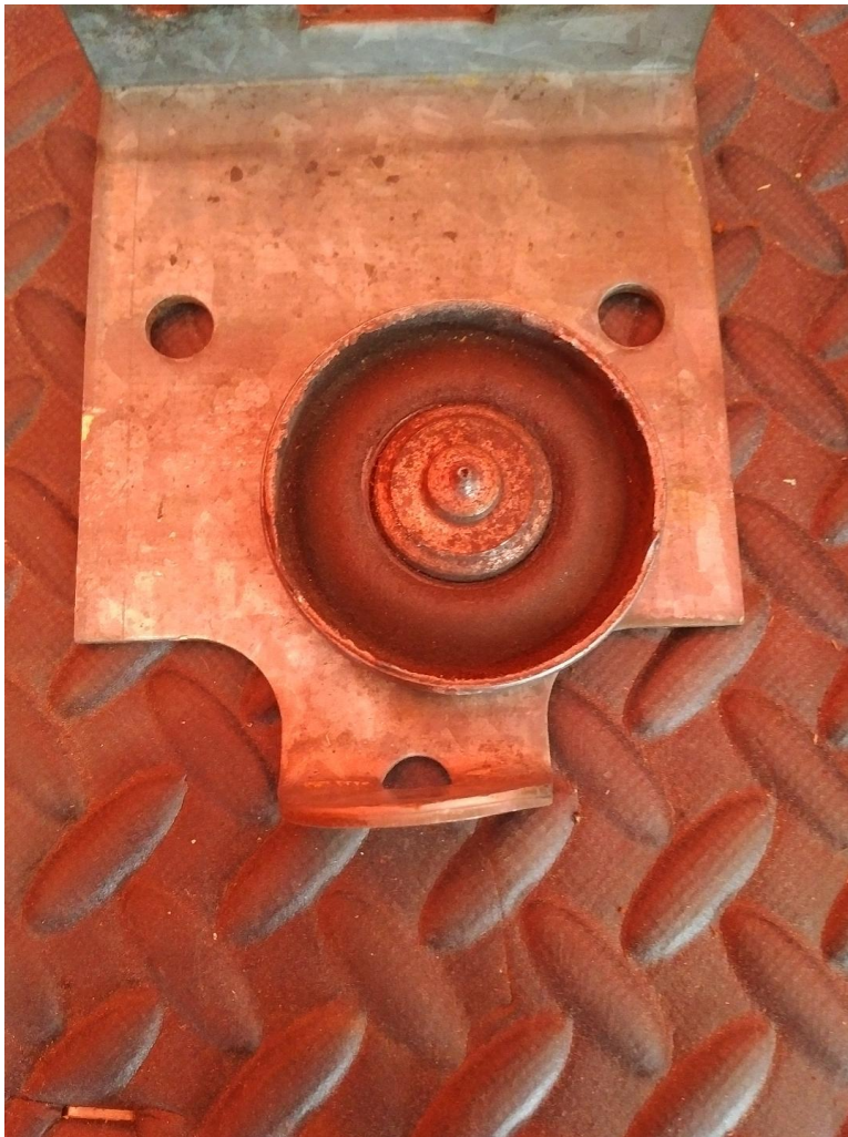
Photo 1: Loose roller completely worn off it's shaft
