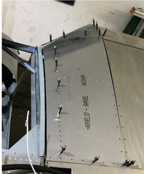
Figure 7. The starboard wing root top skin was fabricated from 6061-T6 donated by Don Walker. This allowed us to make the part to replace the existing one that had mistaken for scrap metal and cut up. Amazingly enough, the rivet holes lined up and we now have a serviceable part.
