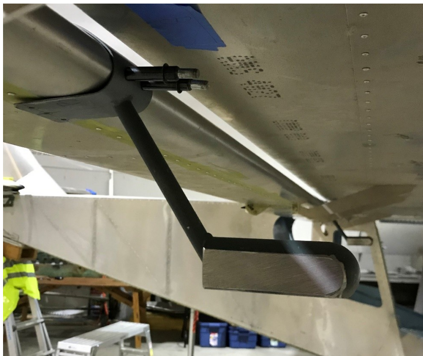
Figure 6. Finished balance weights (apart from a final polish, priming and painting) installed on the starboard wing and sitting in the flaperon neutral position.
