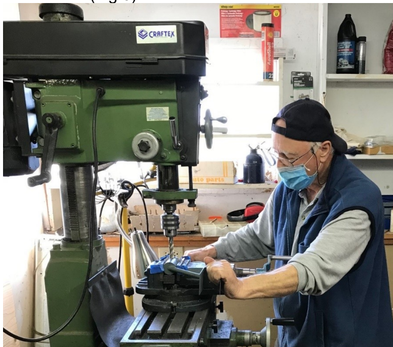
Figure 5. Yves busy with milling one of the balance weights. After getting within 30 gms of the target weight, it then became a repetitive process of testing the weight on the control surface for balance, remove small amounts and then retest.
