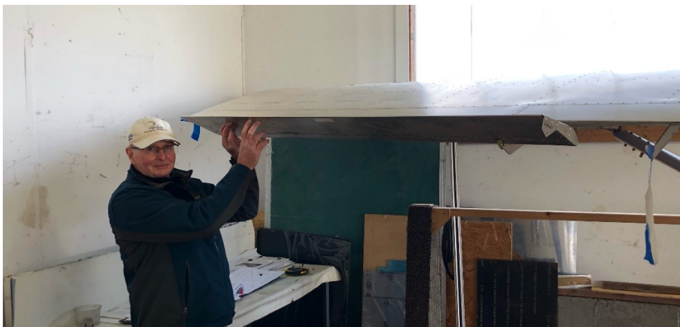
Figure 4. The port aileron installed and supported by two brackets, one near each end that extend from a wing rib through the wing bottom skin. The outboard support bracket for the flap can be seen with a warning ribbon taped to it – these brackets are notorious for walking into!
