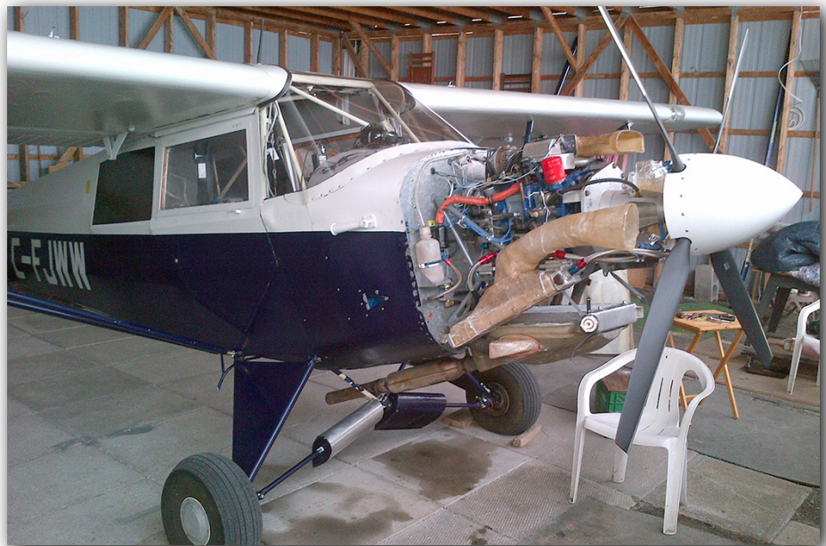
Photo 1: Radiator Install, Flat Profile
