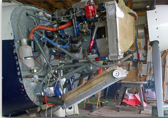
Photo 3: Radiator Install, Tilted Profile
