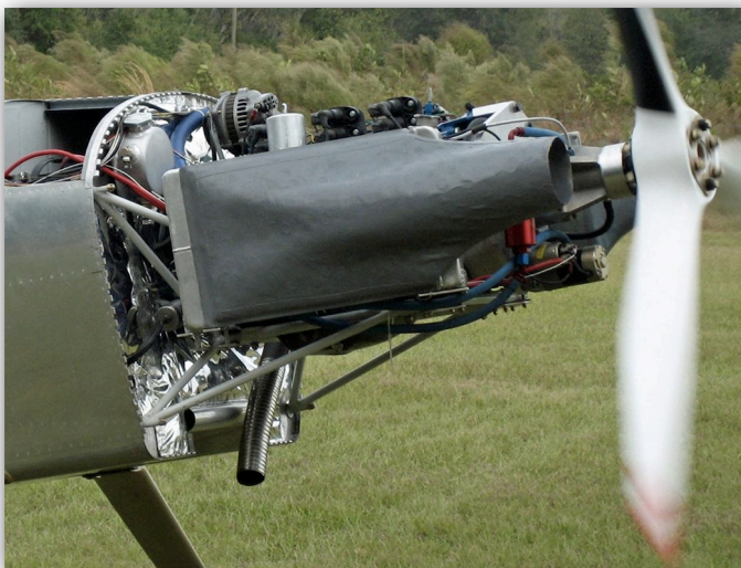
Photo 3: Functional Radiator Install:
