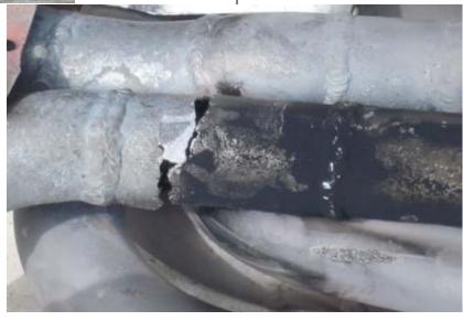
The picture below shows the broken pipe, the remaining pipes on the exhaust system looked great giving no faulty indications. The problem was corrected and C-GMTL is airworthy again. This was not an obvious problem and
