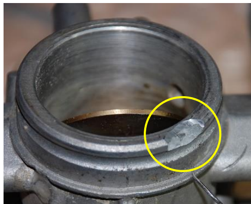
Figure 2. Carb outlet rim with a sharp-edged chip (yellow circle) which would need to be filled and smoothed out.
