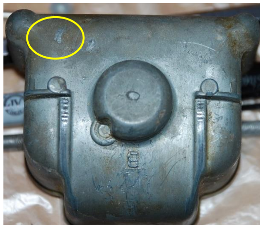
Figure 6. Recent scratches and a minor dent (less than 0.5 mm) are found on the bottom of the fuel bowl (yellow circle).
