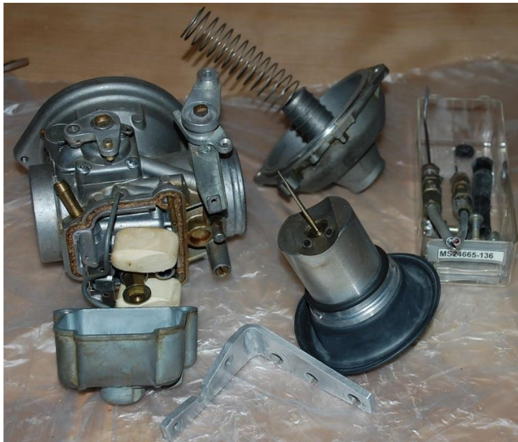
Figure 9. Carb components and straightened cable attachment bracket.
