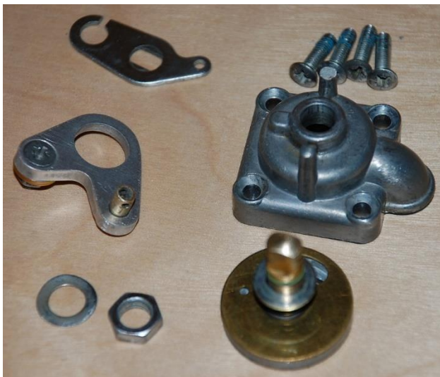
Figure 10. Disassembled choke (left) and throttle (right) assemblies were cleaned prior to reassembly.
