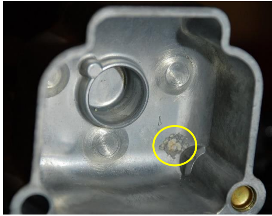
Figure 7. A corrosion patch, 4 to 5 mm in diameter (yellow circle) and just on the surface, has developed in a bottom inside corner of the fuel bowl. This could reflect collected water that sat after fuel had evaporated. The corrosion product was easily removed by scraping and left a smooth, unpitted, surface.
