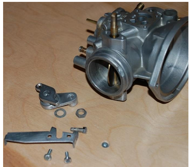
Figure 10. Disassembled choke (left) and throttle (right) assemblies were cleaned prior to reassembly.
