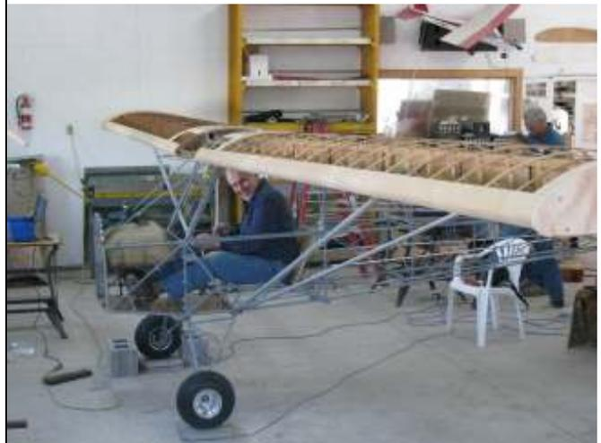
The J3 Kitten is a high wing 3/4 scale J3. It is made up of traditional construction just like the original J3. Chromoly frame, wood wing covered
