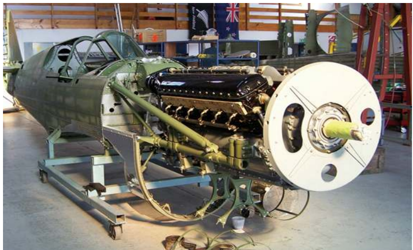
Photo 4 Allison Engine mated to Kittyhawk fuselage by Dave Hadfield
