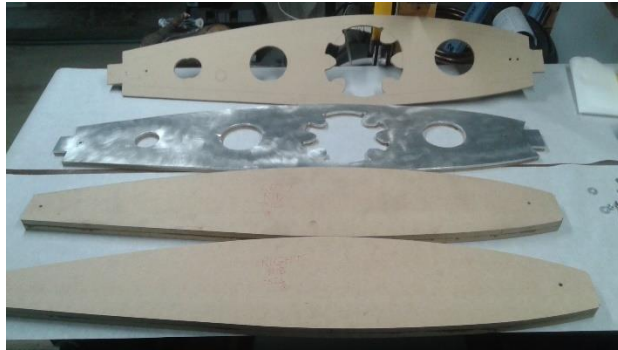
Rib Blank jig and both left and right Flange Bending Jigs
