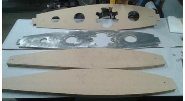
First Rib Blank cut.
