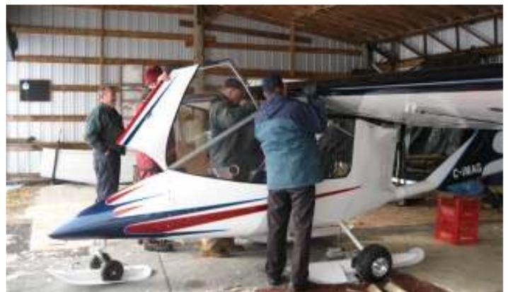
The panel was rearranged to make the radio, transponder and GPS easily reachable. A Dynon PFD was added to supplement the existing steam gauges. Some small adjustment to the rubber seals at the fuselage/wing intersection are still required and then the Titan, will be ready for flight.
