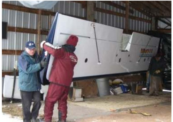
Today we put the wings back on Andre Girard's Titan Tornado. Luckily the temperature was mild. The Titan had a small transformation done to it. A heater and hydraulic skis were added, and the engine motor mount was reinforced as per an AD from Titan.
