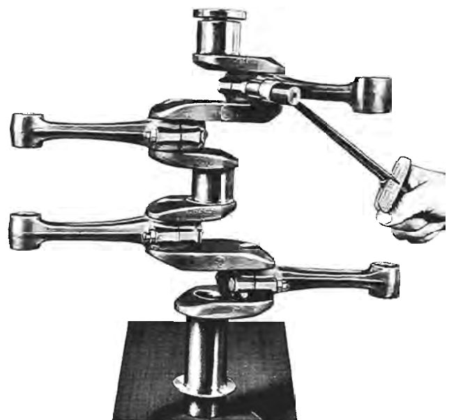
Figure 30. Tightening No. 1 Connecting Rod Bolts.
