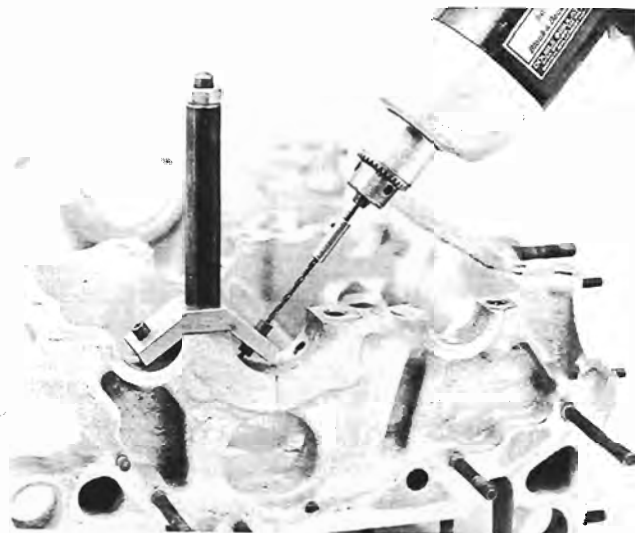
Figure 28. Drill Fixture Installed.
