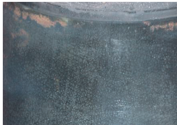
Figure 6-70. Phosphated Cylinder Bore
