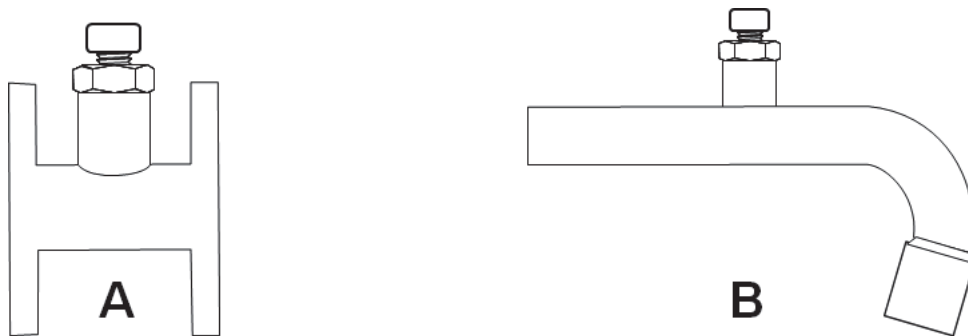
Figure 6-55. Fixed Wastegate (TSIO-520-T) (Typical)
