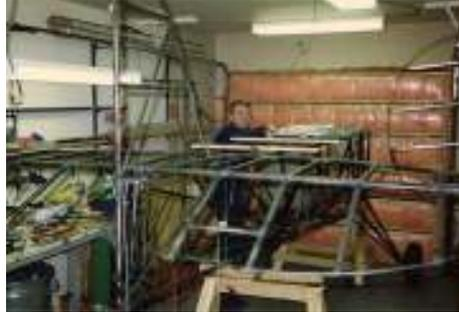
Skybolt 1 Fuselage welding completed
