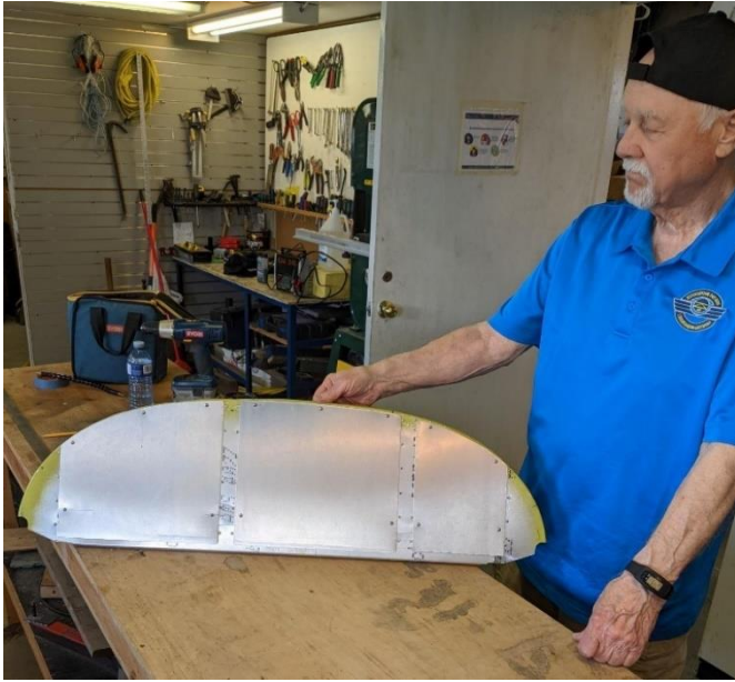
Figure 3. Subpanels fitted to the base panel
