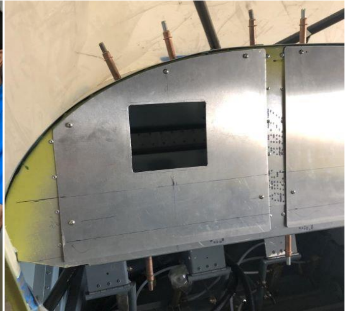
Figure 4. Panel assembly in the Cruiser and the first hole cut for the Dynon D10 EFIS from the old Zenair 601.
