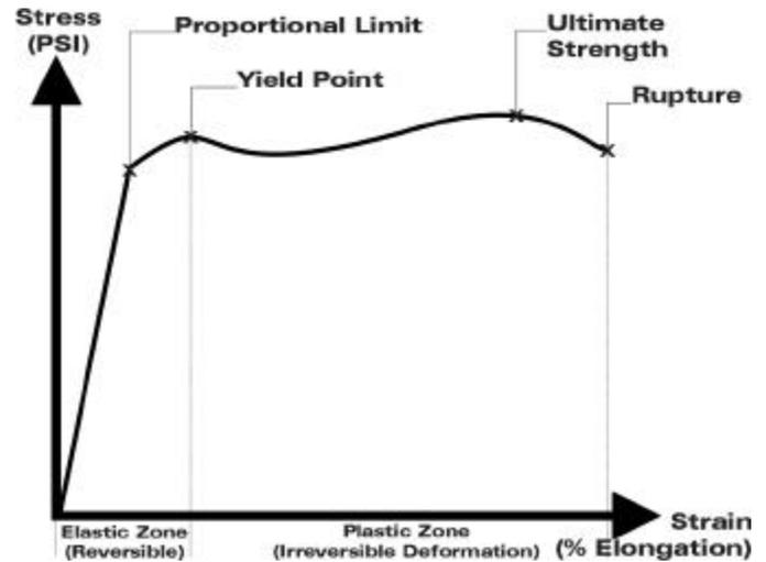
Consider what happens when you apply force to a piece of metal: It deforms. The force you apply is called stress, and the amount of resultant deformation is called strain. The relationship between stress and strain is what defines the structural properties of the metal. (See Figure 4.)
