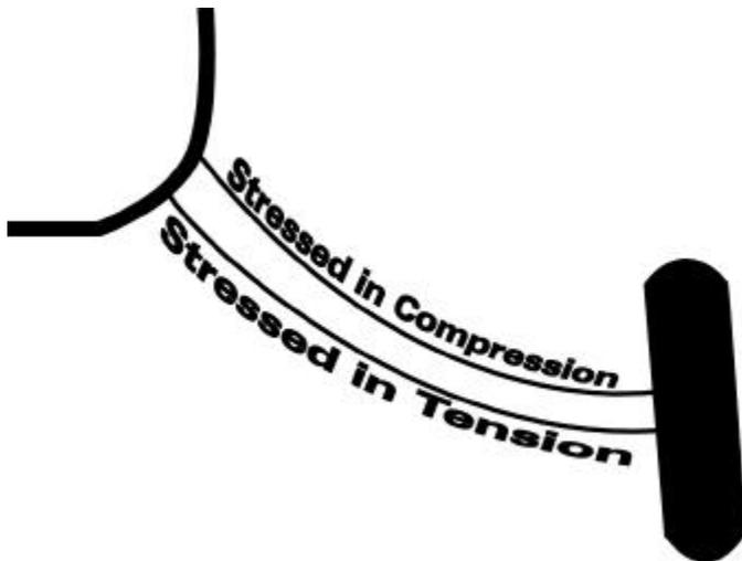
When we think about applying stress to a metal part, we usually think in terms of tension -- in other words, applying a load that tries to pull the metal apart. Cylinder studs and crankcase through-bolts are examples of metal parts that are loaded in tension. Aluminum alloys may have tensile strengths between 20,000 and 80,000 PSI, while high-tensile-strength steel can withstand 200,000 to 400,000 PSI or more.
