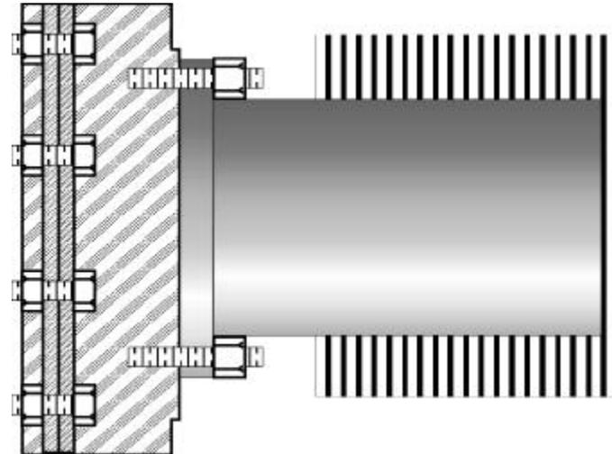
It is crucial for fasteners that undergo cyclic tension loads -- such as crankcase bolts and cylinder hold-down studs -- be torqued properly to ensure that they don't fatigue and fail. Here's why.
