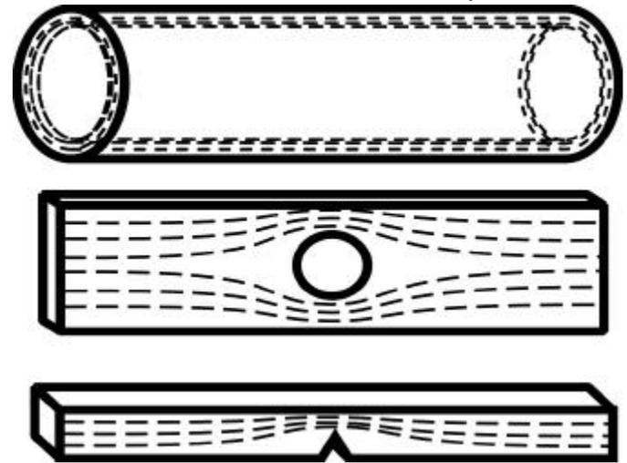
When a metal part is placed under load, stress is almost never uniformly distributed through the part. Instead, it concentrates in certain areas. Naturally, those areas of stress concentration are where the part is most likely to crack or fracture.
