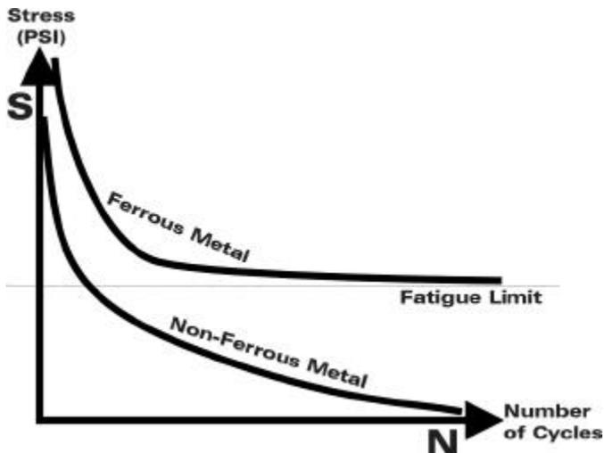
Take an ordinary paper clip, straighten, and then bend it back and forth repeatedly until it breaks in two. What happened? You just demonstrated metal fatigue.
