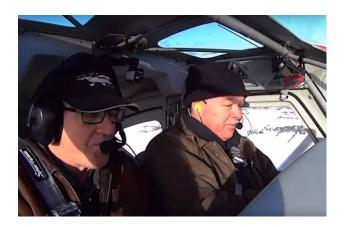
With a new engine to break in our flight profile called for circling near the airport at 75% power, monitoring the engine and staying within gliding distance of the field. The engine ran hard and strong, although maybe a bit thirsty at full rich mixture (this comment coming from a guy who is more accustomed to burning 5 GPH!).
