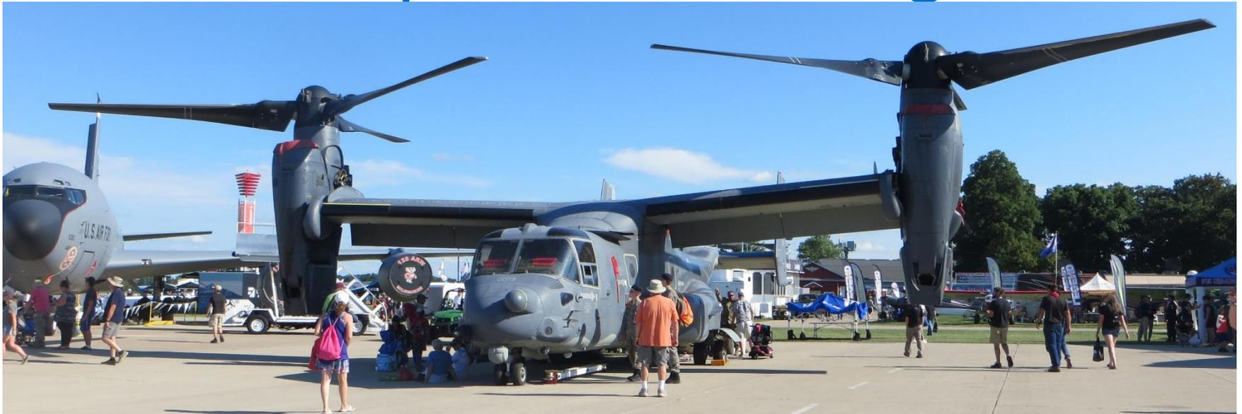
Air Force MV-22 Osprey at Oshkosh 2022. Built by Bell Helicopter Textron, a unit of the Boeing Corp. The Air Force has 54 in Special Operations Command. Two RR Liberty 6200 shaft HP engines, top speed of 280 knots. Crew of 4, armed with 1 .50 cal MG on ramp.
