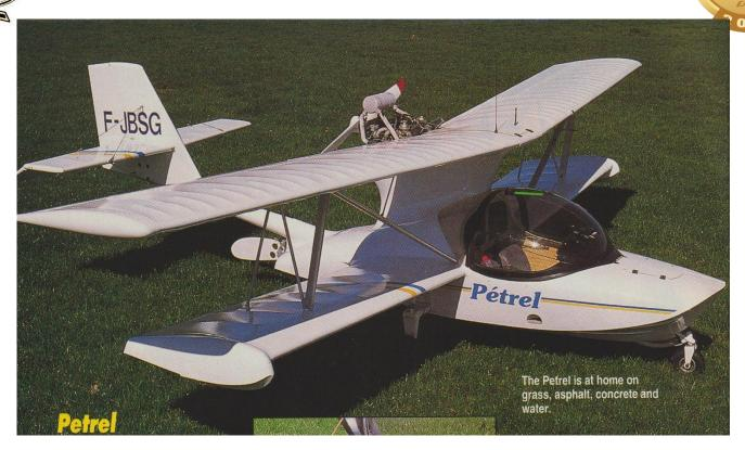
From Kitplanes magazine, Feb 1997 issue. This is the Petrel, French designed biplane amphibian, powered by a Rotax 912 100hp engine. Built of fiberglass, carbon fiber, aluminum, wood and fabric. Kit price from France 24 years ago was \$21,000. Landing gear retracts with a rope and pulley "winding it up" system. Cruise speed is 75 mph, stalls at 35 mph
