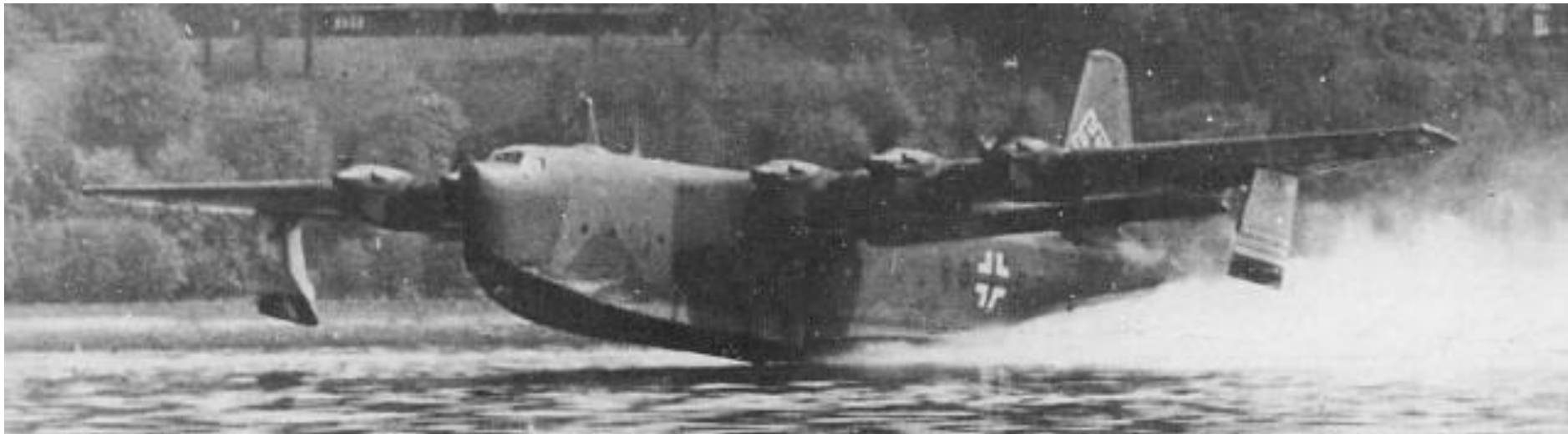
WWII German Blohm & Voss BV 238 Flying Boat – largest aircraft in the world in 1944 at 100 tons takeoff weight. Six 1,750 hp ) Daimler-Benz DB 603 liquid-cooled inverted V12 piston engines
