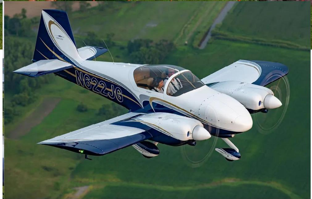
Jim & Ginger Tomaszewski of Clayton, GA converted his RV-6A after flying it 9 years. It uses two Chevy Corvair 6 cylinder engines of 120 HP, with single engine rate of climb at 200 fpm. Cruises at 175 mph, With endurance of 4 hours. New glass Cockpit with autopilot. Really slick!
