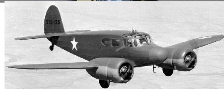
Cessna AT-17/ UC-78 Bobcat from the WASP Museum in Sweetwater, Texas. Used for multi-engine training for future bomber crews. Steel tube and wood construction with fabric covering. Jacobs R-775-9, 245 HP radials. 4600 Bobcats delivered. Nic-named "Bamboo Bomber". Crew of 2, seats for 4. Main gear extended from engine nacelles to minimize damage in gear up landings.
