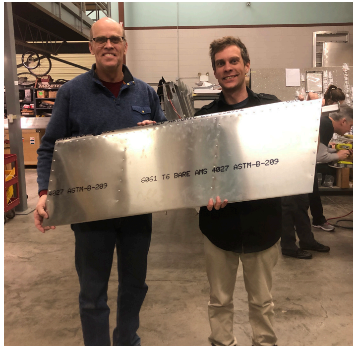
Jay and Nathan holding rudder built at Rans factory training.
