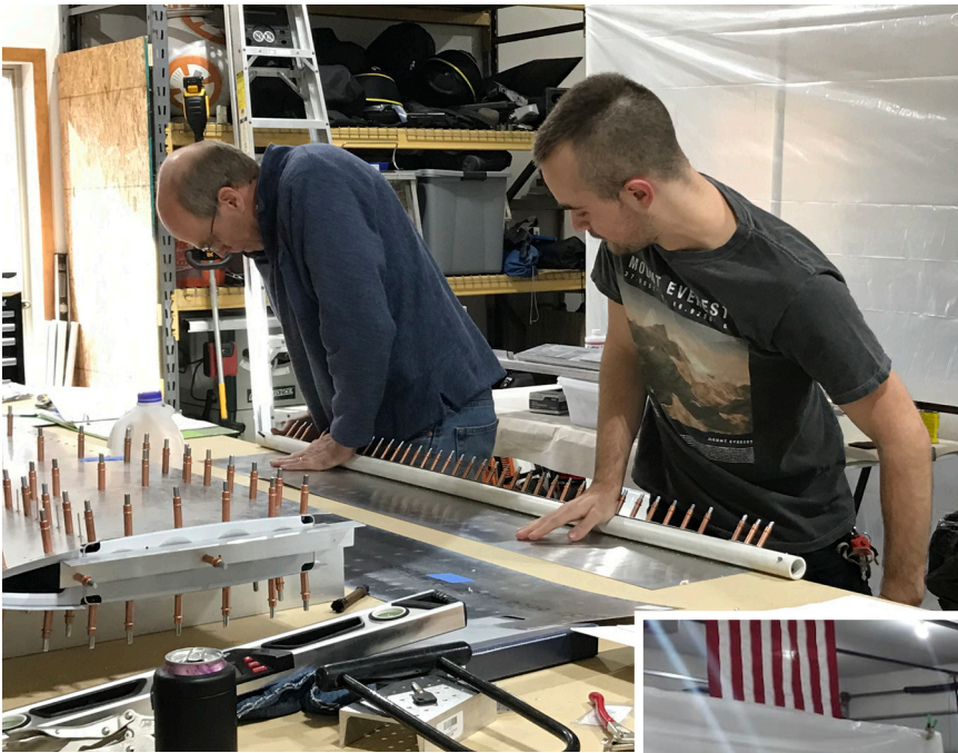
Rolling the aileron leading edge
