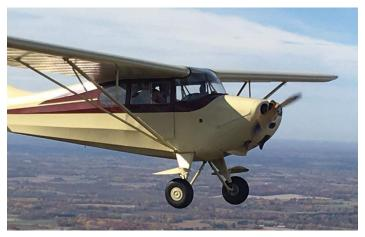
hardware was replaced. Chapter member Dean Griswold and his son, Patrick recovered the wings. Dean took the fuselage up to his place near Princeton, where it was stripped to bare metal, sand blasted and then sprayed with epoxy primer and paint. Then all new wood formers, stringers, and bulkheads were installed. Dean and Bob installed the fuselage covering and then Patrick and Dean finished the coatings and then Dean painted it. The wings were taken to Patrick's
