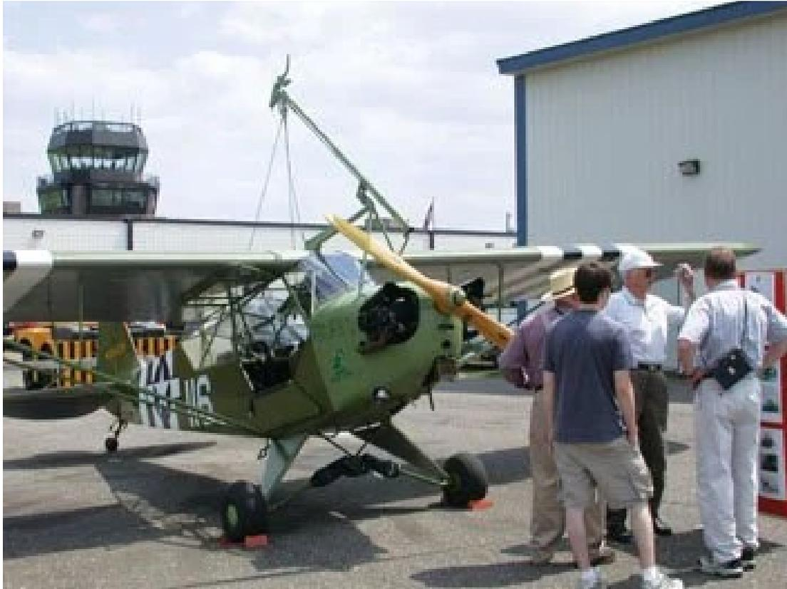
A Piper L-4 Grasshopper demonstrates the Brodie System, in which an aircraft snagged a trolley that ran along a cable in order to land on a short strip or a ship. Caroline Sheen
