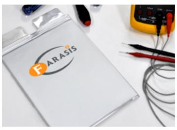
3.65 volt Individual battery cell pouch for 102 volt packs
