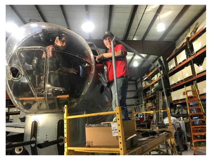
On Monday, January 24, Dick Pugh and I drove over to Oshkosh and met up with Ron Borree of Appleton WI in EAA's Weeks Hangar to replace windows that were damaged in our favorite B-17, "Aluminum Overcast". We brought six curved templates that Dick had made to match the curve of the openings plus tools and Dick's scaffold with us.
