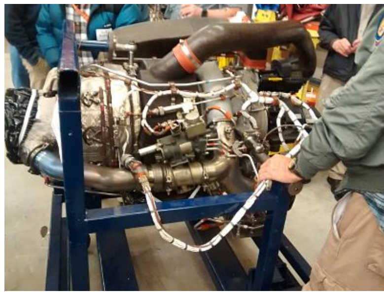
Overhauled Auxiliary Power Unit
