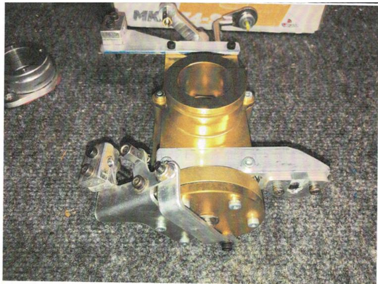
The above Throttle Body Injector is a Rotec TBI MK.II 34-S unit that lists for \$910. Will sell for \$500
