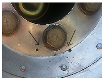
Spinner back plates can be damaged
