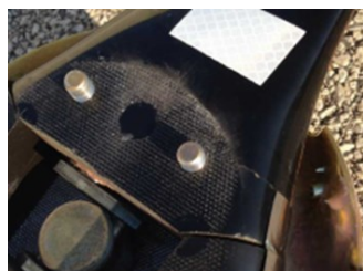
Vibration damage to props can be extremely dangerous
