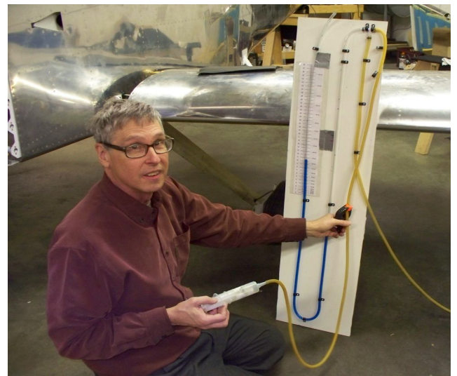
Robert testing the pitot static system for leaks
