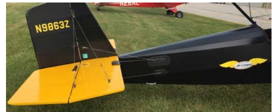
The builder selected a sharp black and yellow paint scheme. He cut pieces from an old leather jacket to protect the horizontal stab and fuselage covering where the control cables exit.
