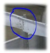
skins off of the fuse last night, quite a few problem rivets, including that the entire rows of rivets along the side stringer or longeron, were of the wrong grip length and didn't really go through the thicker alum angle properly. Very danger-
