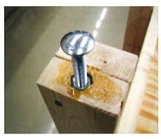
Here we just drilled the hole for the shank of our 1/2-inch carriage bolt. Then drilled a shoulder for the nut. You'll need to use a chisel to conform the hole to the nut and press fit it in. We added a little 5-minute epoxy to keep the nut in place.
